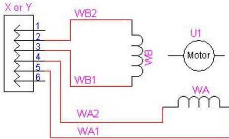
Typical Bipolar Motor Connection
