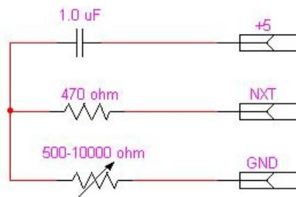
Variable Resistor Circuit for use with PotStepper and UCPotStepper firmware. Selection of the resistance of the potentiometer controls the value range available for the resulting rate generated by the firmware.
