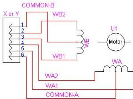
Typical Unipolar Motor Connection
