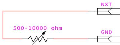
Variable Resistor Circuit for use with PotStepper and firmware when installed on any board which has built-in support for the potentiometer (such as the BS0610M). Selection of the resistance of the potentiometer controls the value range available for the resulting rate generated by the firmware.
