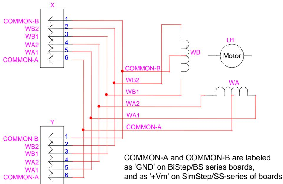
You also will need to have jumper 'R1K' installed, if it is available. If it is not available, you will need to connect a 1K resistor between the RDY output signal and GND.
