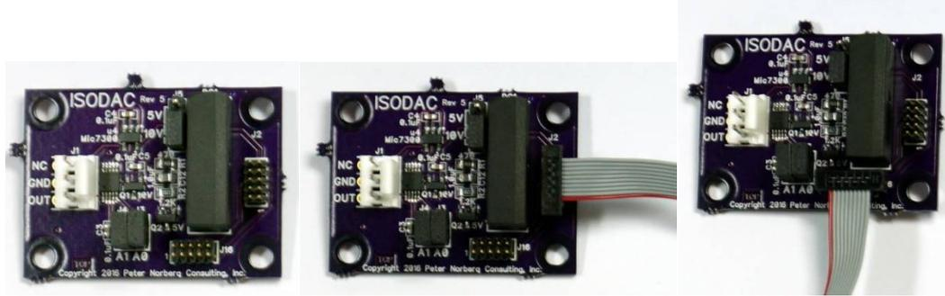
The image on the left shows the revision 5 board, the one in the center shows board with a JTAG cable attached to the rightmost connector, and the one on the right shows the board with the JTAG cable attached to the bottom connector. The white connector on the left is the Amp MTA-100 connector (which may be replaced with a screw terminal connector as an order option) that provides the output signals from the board.
